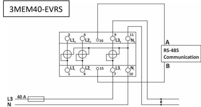
Figure 2: Single-phase connection diagram
